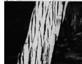
Fig. 5.80 Massive \alpha in an Fe-0.002 wt% C quenched into iced brine from 1000 °C. (book, 8th)
