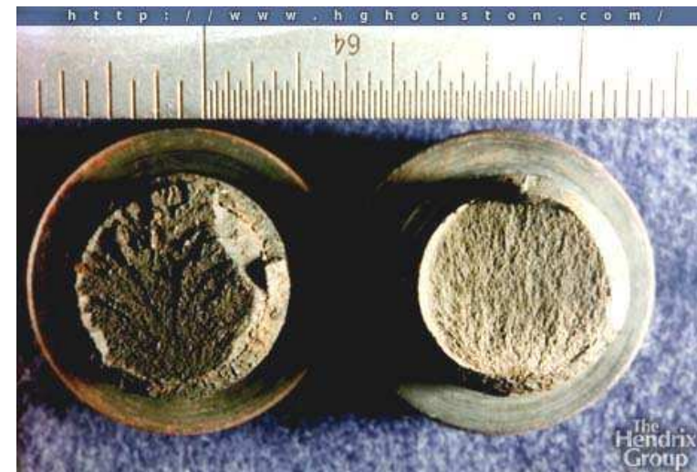
Hydrogen Embrittlement of Valve Capscrew Fasteners – Source: The Hendrix Group
