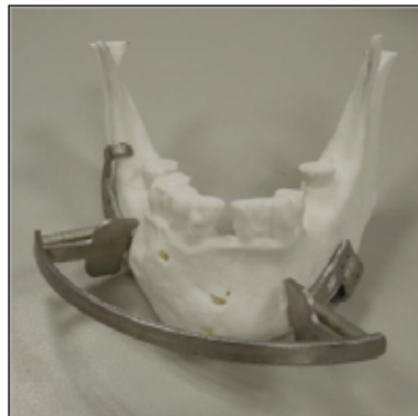
316L Surgical guide made by Laser Beam Melting (Courtesy of IK4-Lortek)
