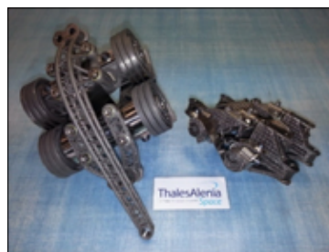
Solar panel deployer for satellite made by SLM in 3 parts (right) vs 25 parts (left) with conventional manufacturing (Courtesy Thales Alenia Space and Poly-Shape)
