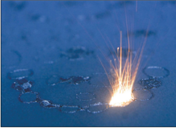
Laser beam melting operation (Courtesy of EOS)
