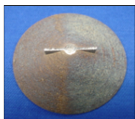
Staircase effect (Courtesy of Fraunhofer IFAM)
