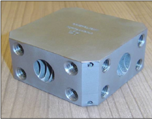
Hydraulic prototype with complex internal channels, (Source: EU project COMPOLIGHT)
