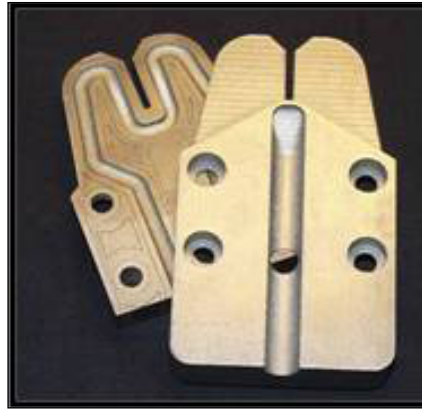
Tooling insert by Laser Beam Melting (Courtesy of BMW)
