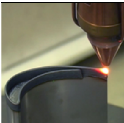
Direct Energy Deposition process for blade repair or building (Courtesy of Fraunhofer ILT)
