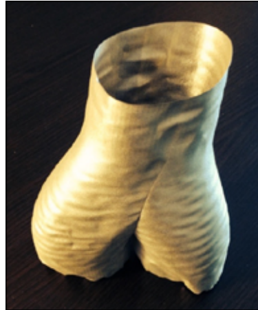
Ni718 manifold showing buckling effect due to too thin walls (Courtesy of Renishaw)
