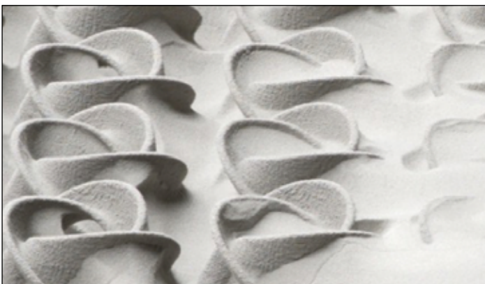
Parts in the powder bed after 3D printing (Courtesy of Höganäs AB - Digital Metal®)
