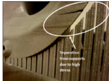
Part distortion due to residual stresses leading to the separation of part from supports (Courtesy of Renishaw)
