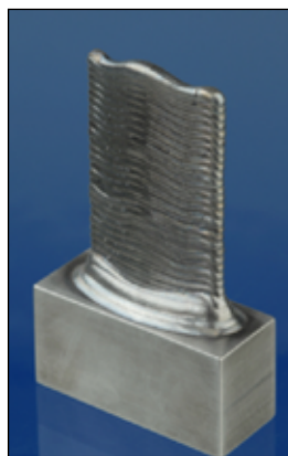
Direct Energy Deposition process for blade repair or building (Courtesy of Fraunhofer ILT)
