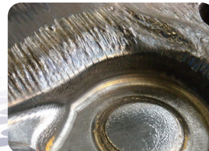
Tool wear white lubricant 6500 strokes
