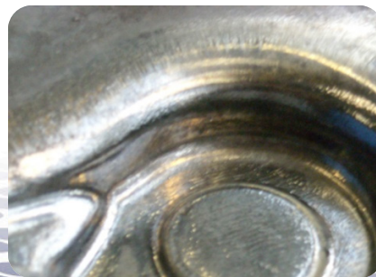
Tool wear graphite lubricant 15000 strokes
